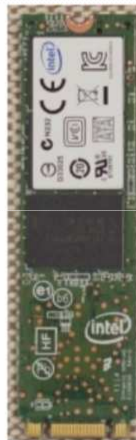
B/M keyed SSD using the PCIe x2 bus
