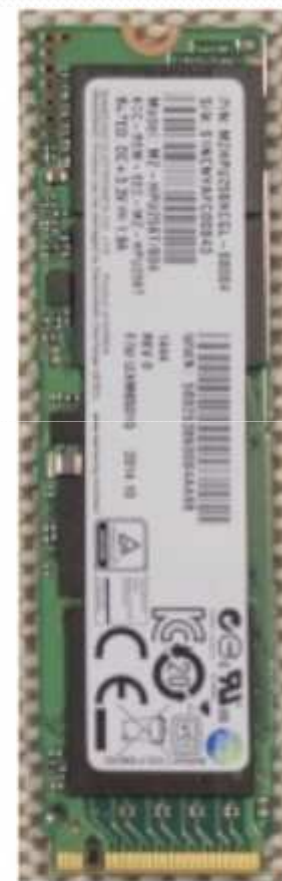
M keyed SSD using the PCIe x4 bus
