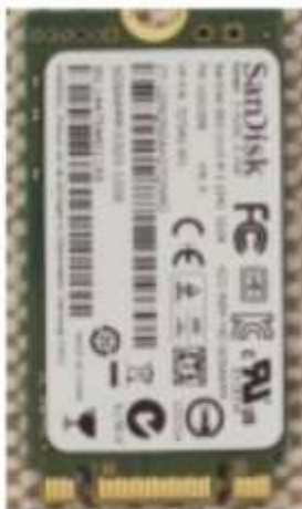
B/M keyed SSD using the PCIe x2 bus
